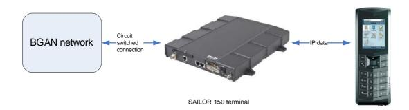
When connected to the terminal the IP handset provides a dedicated BGAN menu with a subset of the terminal configuration options.
